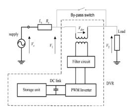
Fig1. Typical DVR connected distribution system.
