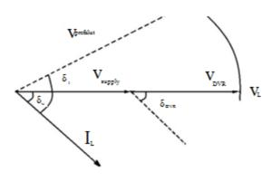
Fig 4. In-phase compensation method
