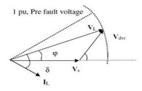
Fig 5. Phasor diagram of minimal energy technique
