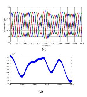
Fig .8. (a) supply voltage  $V_s$ , (b) injected voltage  $(V_{dvr})$ , (c) load voltage  $(V_l)$ , (d)DC component of injected active power,  $(P_{dvr,dc})$
