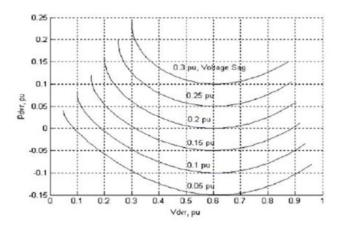
Fig 6 injected active power vs injected voltage
